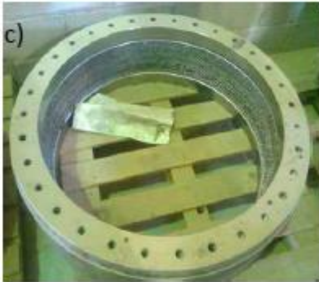
Equipment used for pelletization: a) milling unit; b) pelletization unit; c) press die; d) pellet cooling reservoir
